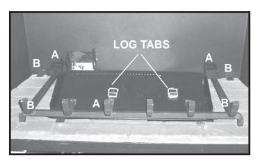
**STEP 1:** Remove metal grate supports (A) and refractory tabs (B) by using a back and forth motion until the tabs break free. Metal tabs and supports are needed for shipping only. After removing the tabs and supports, the grate should fully rest on the base refractory.
